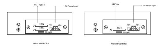
Note: standard package only supports single SIM, dual SIM is an optional feature.
